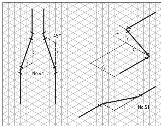
Changes of direction are shown in the ratio of 2:1 or 1:2 irrespective of angles and dimensions. By drawing in the triangle as an aid the change of direction is set accurately. The divergence is established by giving the type of fitting (catalogue no. or angle) or by dimensioning.
