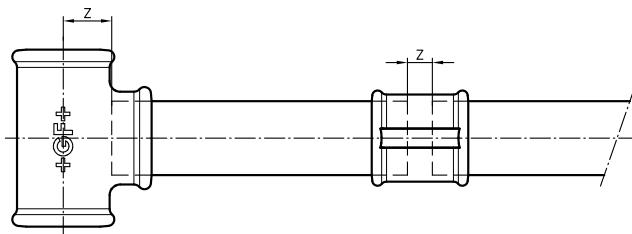
The z dimensions are calculated from the overall lengths less the average length of engagement. z dimensions were introduced by Georg Fischer to support the rational planning and preparation of work.
