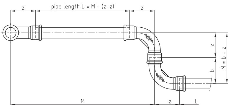
Exact pipe thread lengths produce exact  $M$  dimensions.
