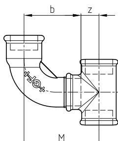
For fittings combinations with internal and external threads the distance of the axes arises from adding  $z + b$ :
