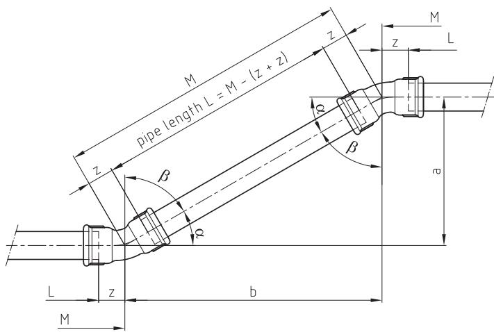
The  $M$  dimension for sloping pipe sections can easily be calculated by using the factor table or the numerical table.
