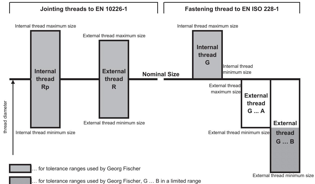
illstr. 1 Tolerances of jointing and fastening threads
