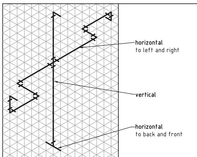
Pipelines sloping in relation to each other are drawn as shown in the example below:
