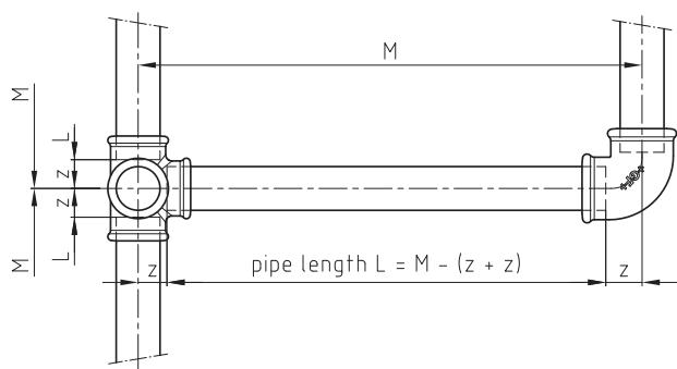
Principle of the  $z$  dimension method: consistent method of measuring centre - centre =  $M$
